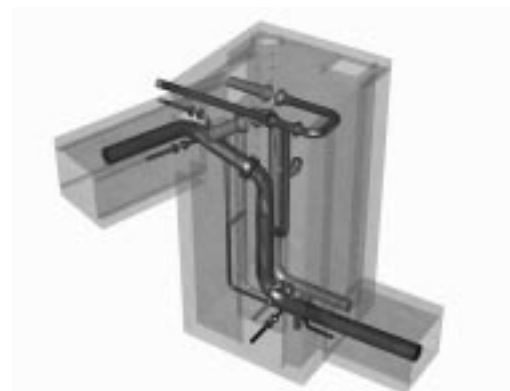
Steam Distribution Manhole Model
