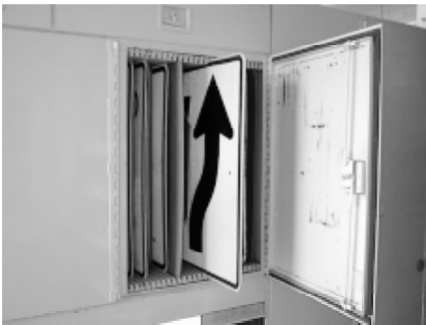
Truck storage compartment for completed signs
