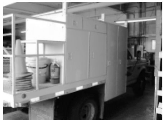
Sign storage cabinets on medium-sized truck
