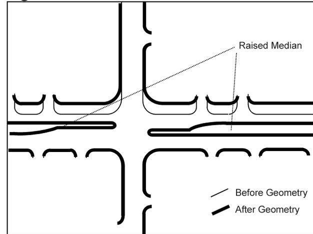
**Figure 48—Left turn lanes with continuous raised median**
