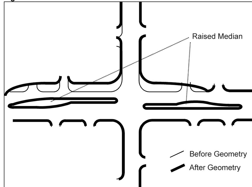
**Figure 47—Left turn lanes with continuous raised median**
