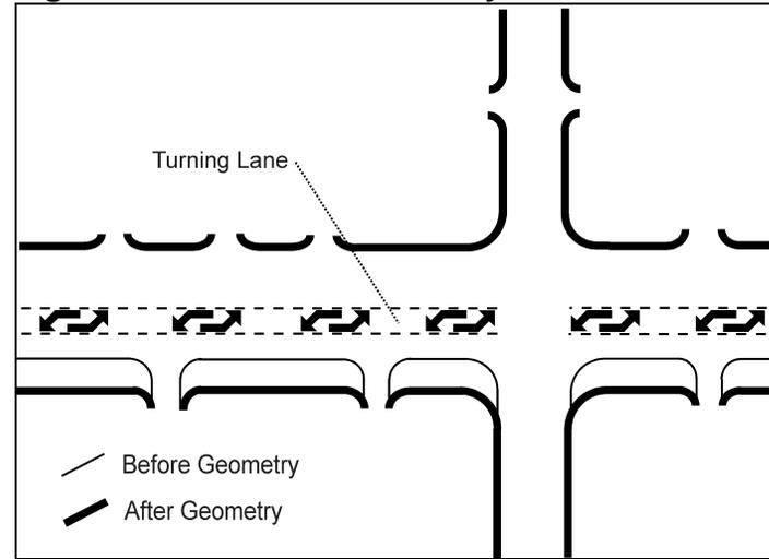
**Figure 50—Continuous two-way left turn lane**
