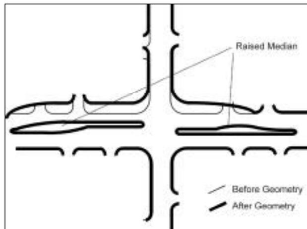
The above retrofit project shows the installation of a raised median with left-turn lanes at an intersection. The project was conducted in conjunction with a program for managing access to driveways located within the functional area of the intersection. In this example, some driveways were closed, consolidated, and cleared away from the intersection.
