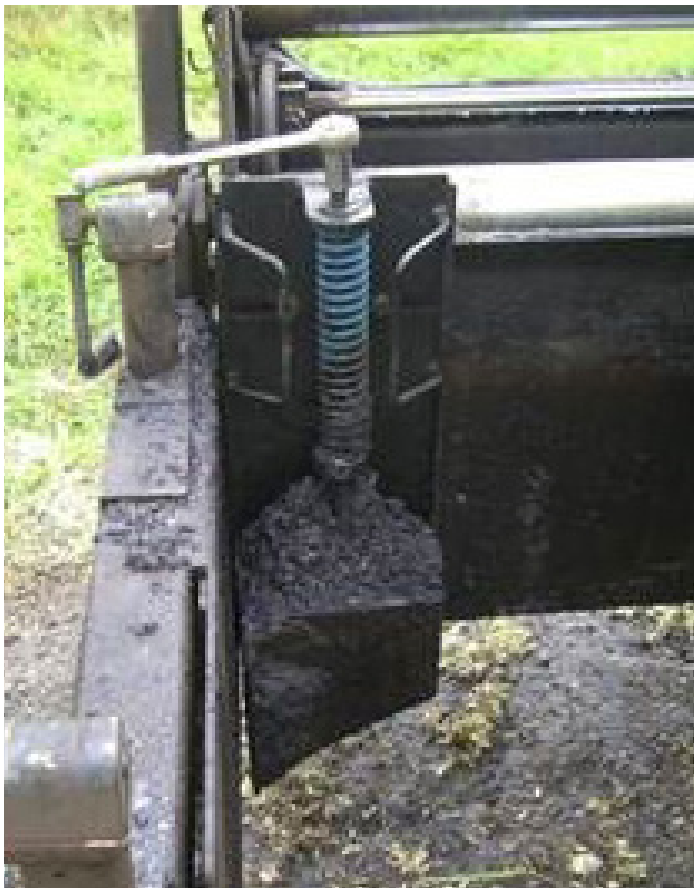
Advant-Edger, an adjustable, reversible attachment that can be mounted on either side of the paver, designed to create a well defined and durable 30° Safety Edge
