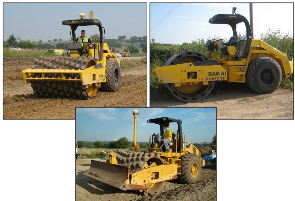
Figure 1. Sakai SV610 padfoot roller (left), Sakai SV610 padfoot roller setup with smooth drum shellkit (right), and Caterpillar CS56 padfoot roller (bottom)
