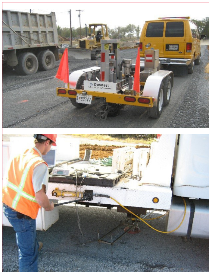
Figure 2. Dynatest FWD (top) and static plate load test (bottom)
