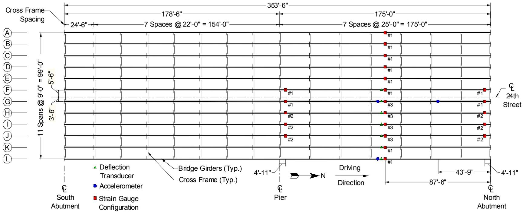
Figure 4.15. Gauge location on bridge
