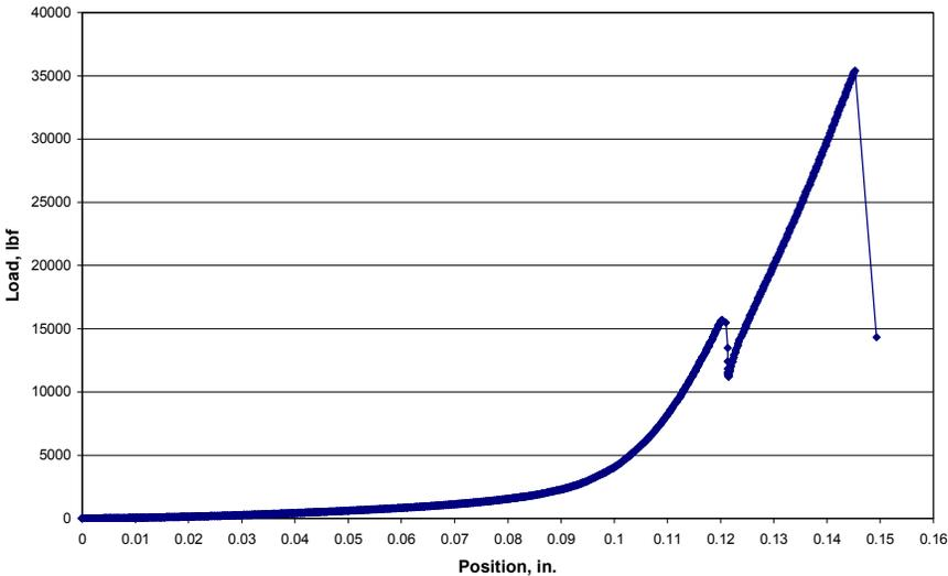
**Figure 3.4. Deflection vs. Load plot for sandblasted specimen #3**
