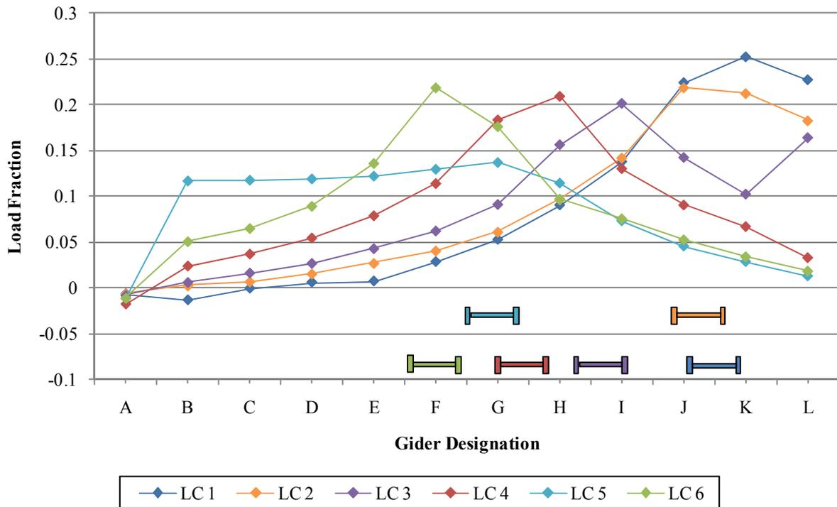
**Figure 4.26. Experimentally-obtained load fraction for six load cases**
