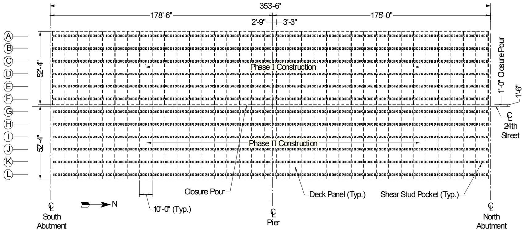
Figure 2.6. Precast panel layout
