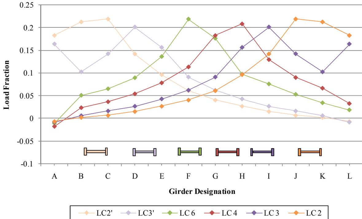
Figure 4.27. Load fractions combined to form load distribution
