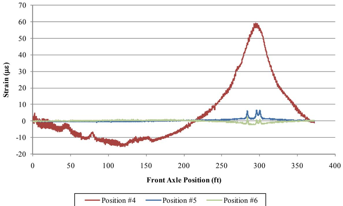
**Figure 4.23. Girder J cross-section strain, Load Case 2**
