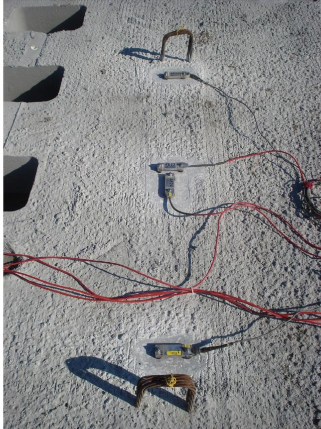
**Figure 4.7. Strain gauge orientation for each gauge line**
