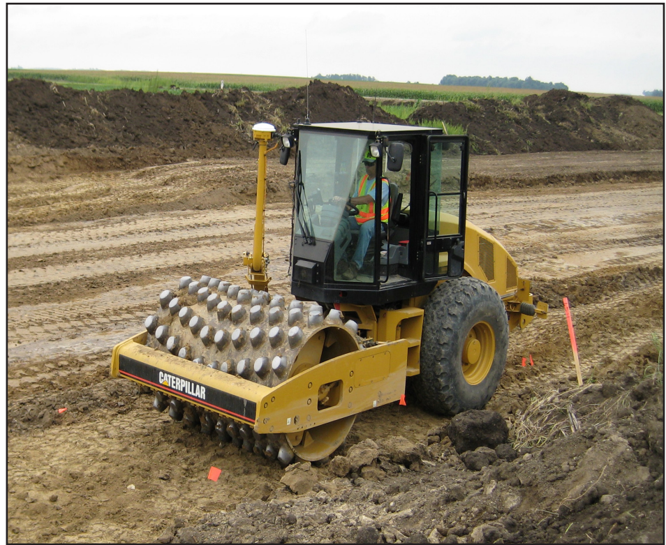
Figure 1. Caterpillar CP563 padfoot roller with MDP* measurement system on TH 60 project (from White et al. 2009)
