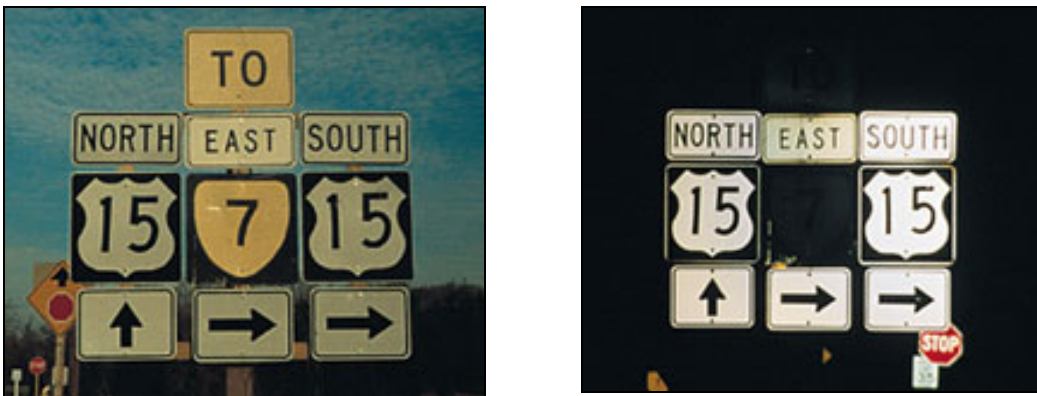
Figure 6. Illustrates loss of retroreflectivity at night (Image source: Opiela et al. 2003)
