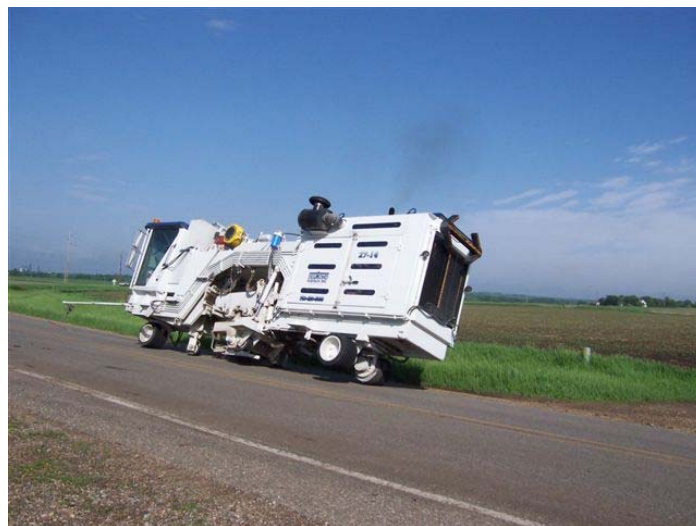
Figure 3-11. Machine tipping on inside curve
