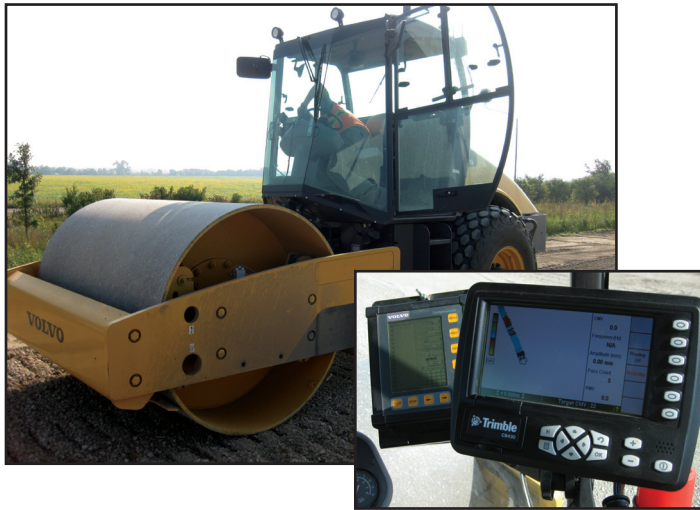
Figure 1. Volvo SD116DX smooth drum vibratory roller (top), and the onboard Trimble CB430 display (bottom) (from White et al. 2010)
