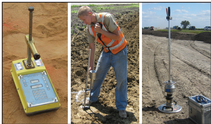
Figure 2. Nuclear gage (top left), dynamic cone penetrometer (top right), light weight deflectometer (bottom) (from White et al. 2010)
