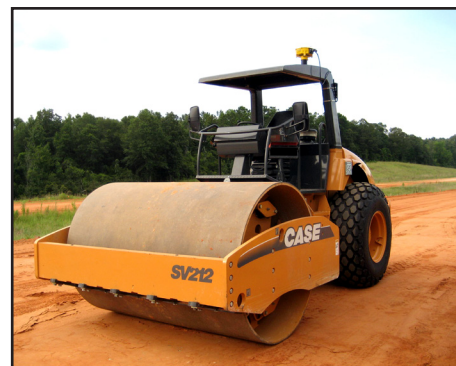
Figure 1 – Caterpillar CP56 (top left) padfoot roller equipped with MDP technology, Case SV212 (above) smooth drum roller equipped with k technology, and Sakai SW880 (bottom left) dual smooth drum roller equipped with CCV technology (from White et al. 2010)
