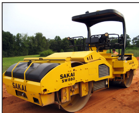
Figure 1 – Caterpillar CP56 (top left) padfoot roller equipped with MDP technology, Case SV212 (above) smooth drum roller equipped with k technology, and Sakai SW880 (bottom left) dual smooth drum roller equipped with CCV technology (from White et al. 2010)
