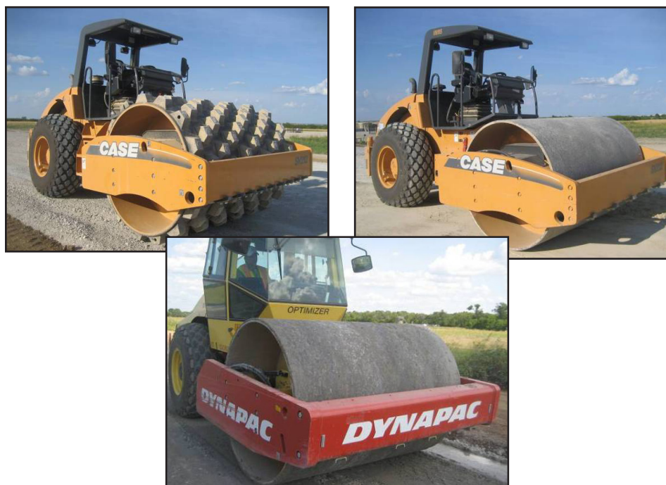
Figure 1. (left) Case SV212 padfoot roller, (right) Case SV212 smooth drum roller, and (bottom) Dynapac CA362 smooth drum roller
