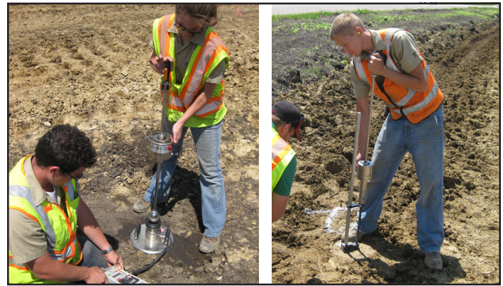
Figure 2. Light weight deflectometer test (left) and dynamic cone penetrometer test (right) (from White et al. 2010)
