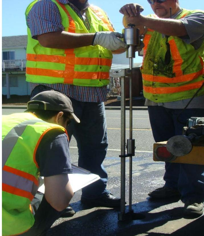
Figure 4.8: Photos of Dynamic Cone Penetrometer Testing
