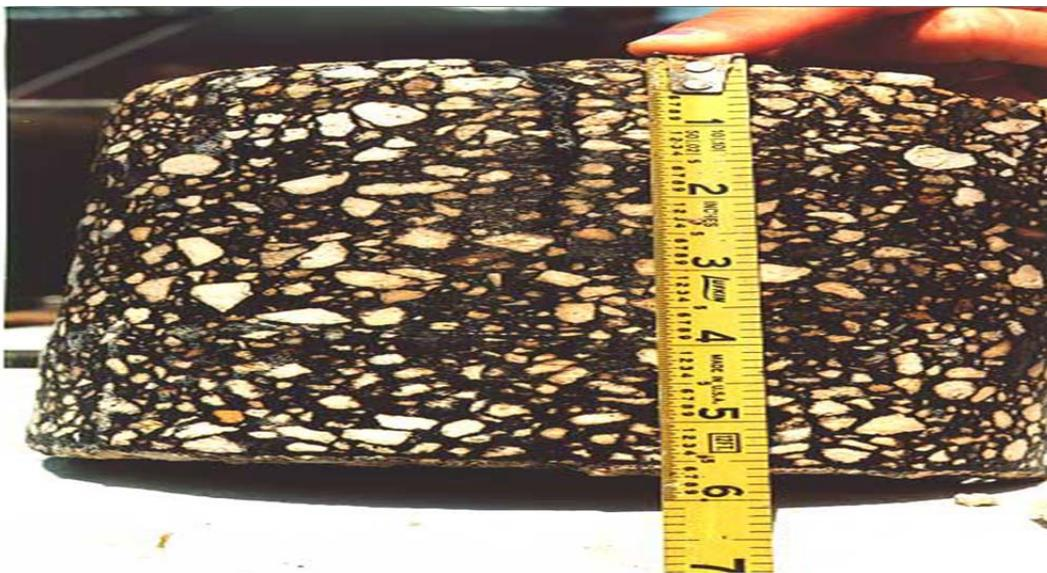
Figure 2.2: Core Extracted from Wheelpath Shows Top-Down Cracking (Myers et al. 2001)
