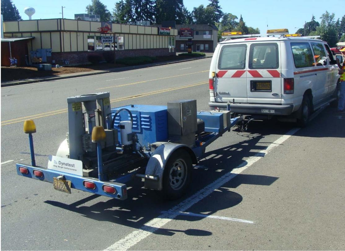
Figure 4.5: FWD Testing Used by ODOT
