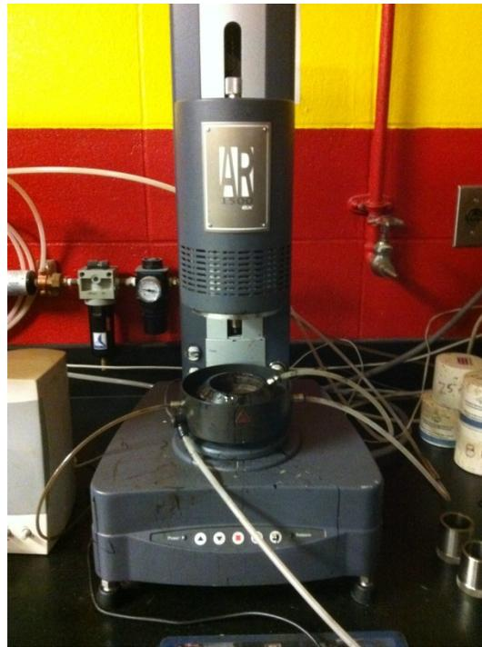
Figure 4.16: AR1500 Dynamic Shear Rheometer
