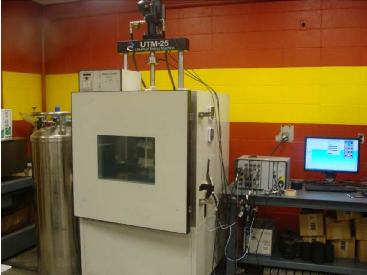
Figure 4.11: UTM-25 Machine for Dynamic Modulus Testing
