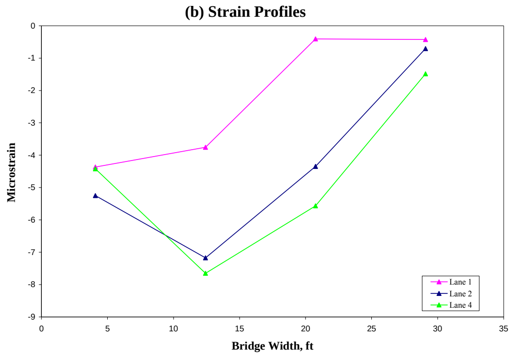
Figure 3.3 MS 2 Strain and Deflection Profiles (Load Case 2)
