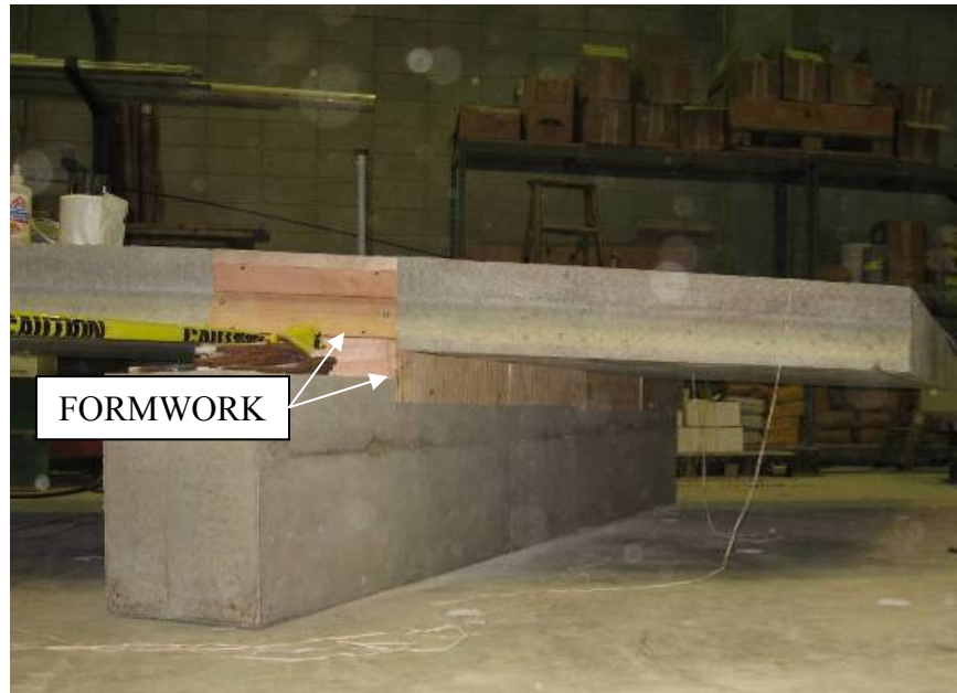
a) Formwork along bottom of channel
