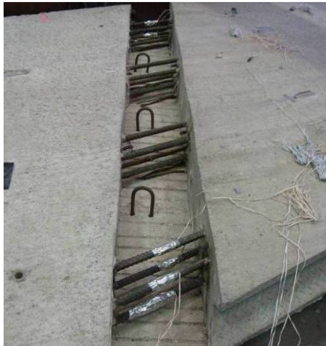
Figure 2.10. Reinforcing bars instrumented with steel strain gages
