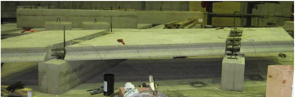
Figure 2.14. Deck panel setup for leveling test
