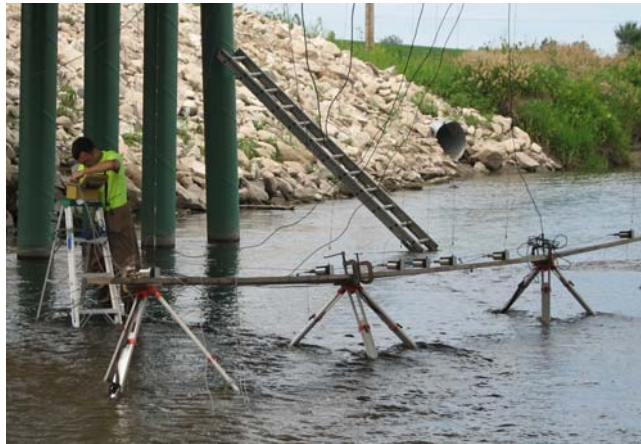
Figure 2.3 Tripod system used to support displacement transducers
