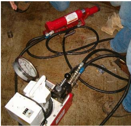
a) Mono-strand jack and hydraulic pump
