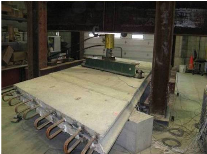
Figure 2.26. Laboratory setup for Panel 3 ultimate load test
