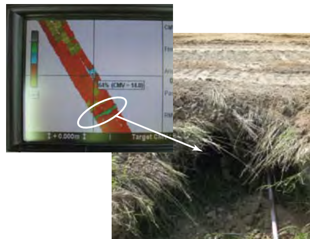
Figure 7. CMV map on an on-board display highlighting a box culvert location with a high CMV
