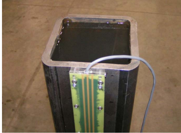
Figure 4.3. Image of sensor array and water-filled test pile
