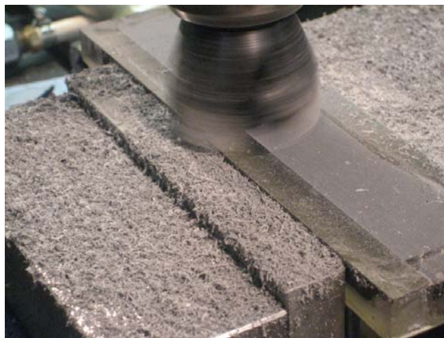
Figure 3.9. Photograph of the milling operation to level epoxy
