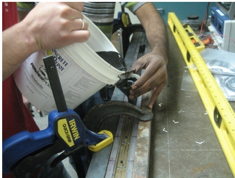
Figure 3.12. Pouring epoxy into large test array
