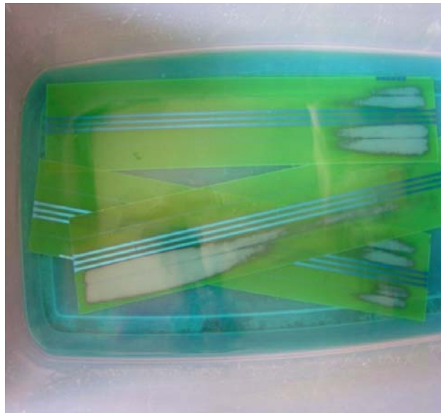
Figure 3.7. Excess copper being removed from the printed board
