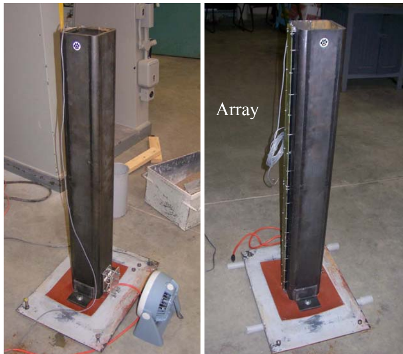
Figure 4.2. Both sides of large test pile, showing heater and array locations
