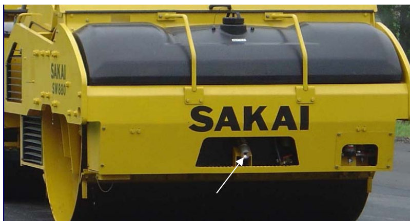
Figure 6. Photograph showing infrared temperature sensor on the RICM roller to measure HMA surface temperature (Courtesy of Sakai)
