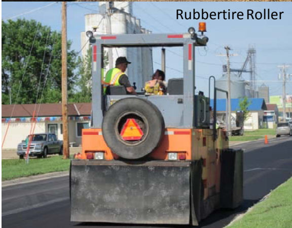
Figure 81. Breakdown, rubbertire, and finish rollers equipped with Topcon's on-board display unit – IA9 Kossuth/Winnebago County project construction
