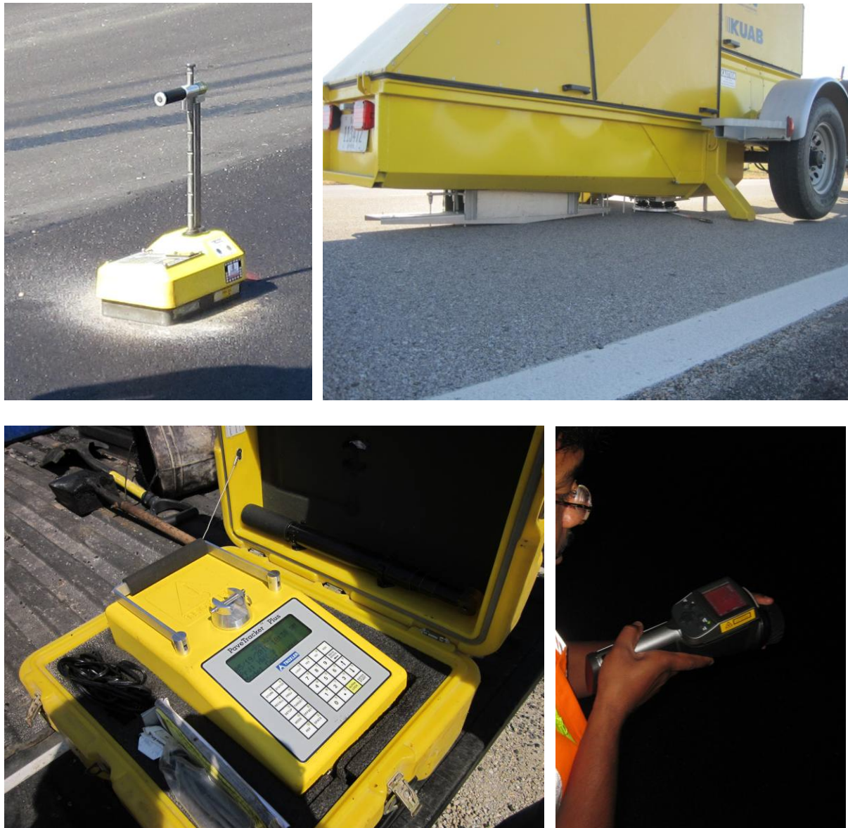
Figure 1. In-situ testing methods used on the project: Humboldt nuclear gauge (top left), Kuab falling weight deflectometer (top right), Pavetracker non-nuclear density gauge (bottom left), and Flir thermal imaging camera (bottom right)
