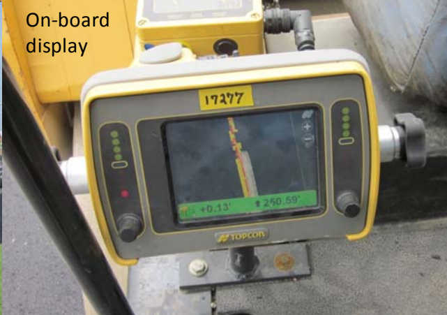
Figure 81. Breakdown, rubbertire, and finish rollers equipped with Topcon's on-board display unit – IA9 Kossuth/Winnebago County project construction
