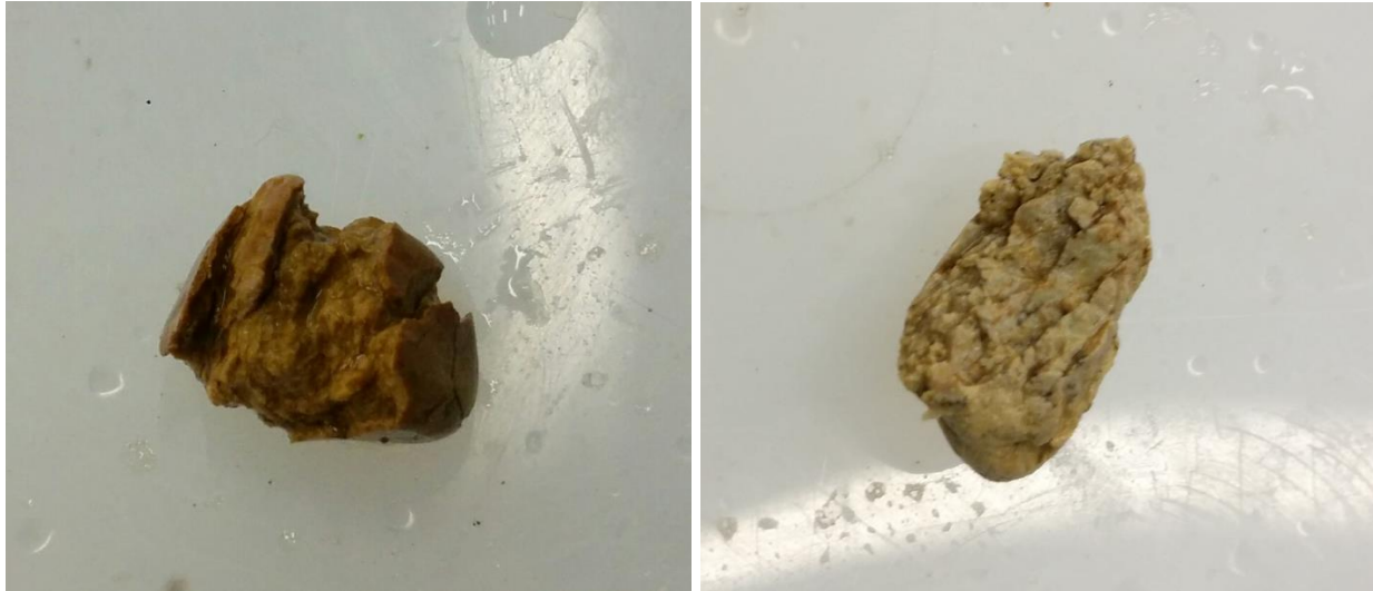
Figure 5. Fraying after freezing-thawing cycles in the CSA A23.2-24A test (1/2 inch aggregate particles)
