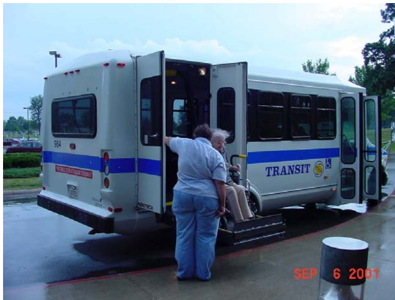
Figure 22. Light-duty bus equipped with wheelchair lift in conformance with ADA accessibility standards (courtesy of Region 15)
