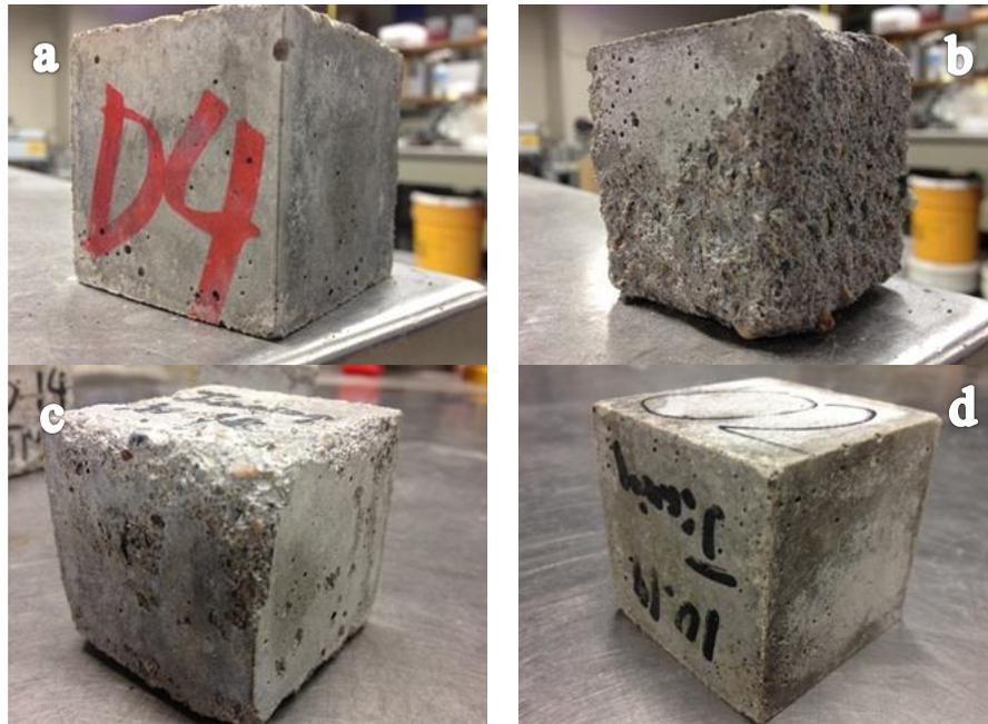
**Figure 7. Condition of cubes after 10 freezing-thawing cycles: a) plain water, b) 3% sodium chloride, c) 4% calcium chloride, d) Ossian Season One**
