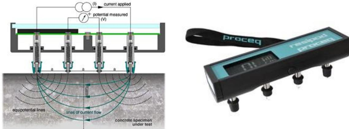
**Figure 4. Wenner array probe for electrical resistivity measurement**
