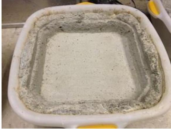
**Figure 2. Concrete slab for scaling evaluation**
