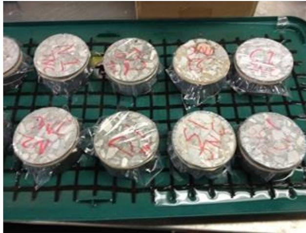
**Figure 6. Water absorption specimens**
