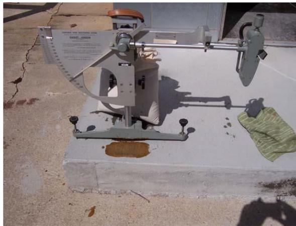
**Figure 3. British Pendulum for skid resistance**
