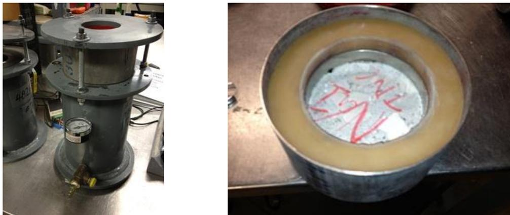
**Figure 5. Air permeability apparatus and test specimens sealed tight at the perimeter**
