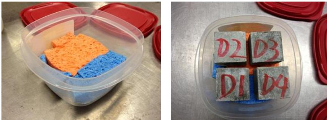
**Figure 1. Test cells for cyclic freezing and thawing**
