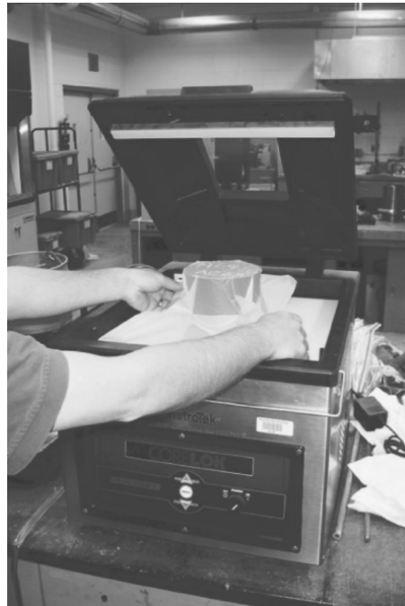
Figure 3. CoreLok Vacuum Sealing Device (Buchanan and White 2005)
