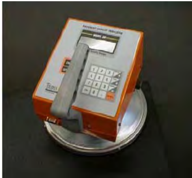
Figure 5. Pavement Quality Indicator (TransTech 2002)
