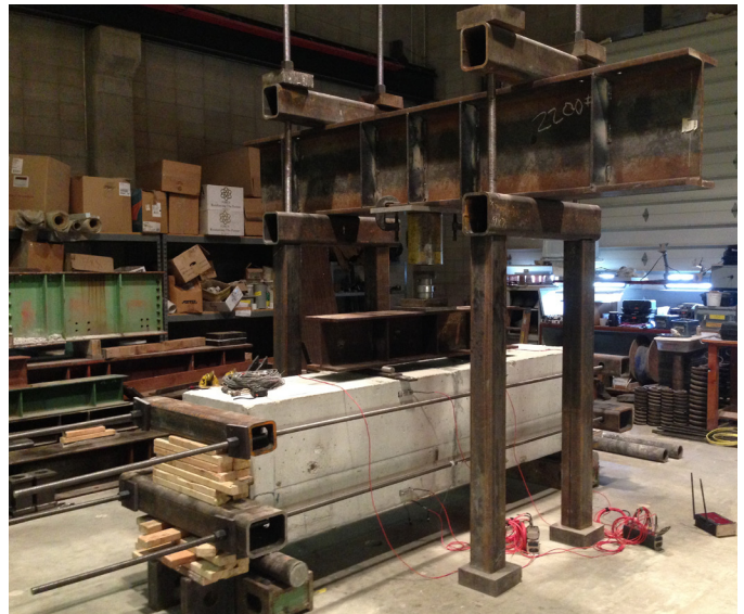
Static four-point bending test with applied axial load: specimen in the test frame setup with axial load applied with post-tension rods
