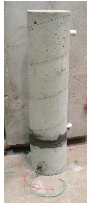
Small grouted coupler specimen for chloride penetration testing after grouting
