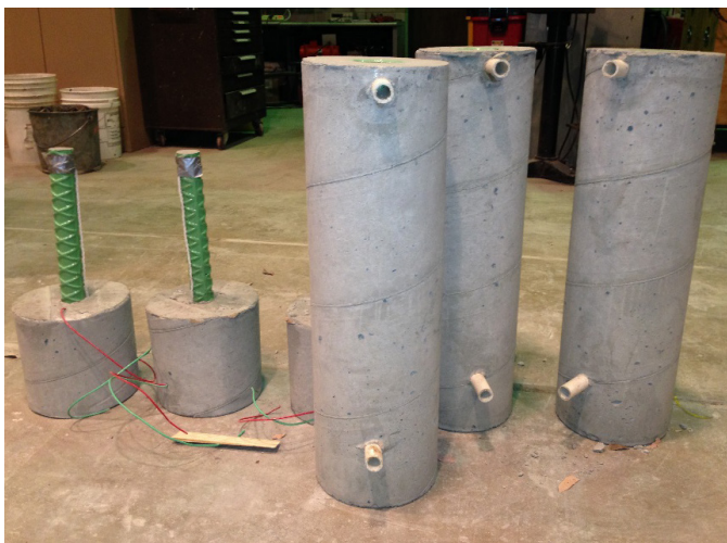
Small grouted coupler specimens for chloride penetration testing prior to grouting
