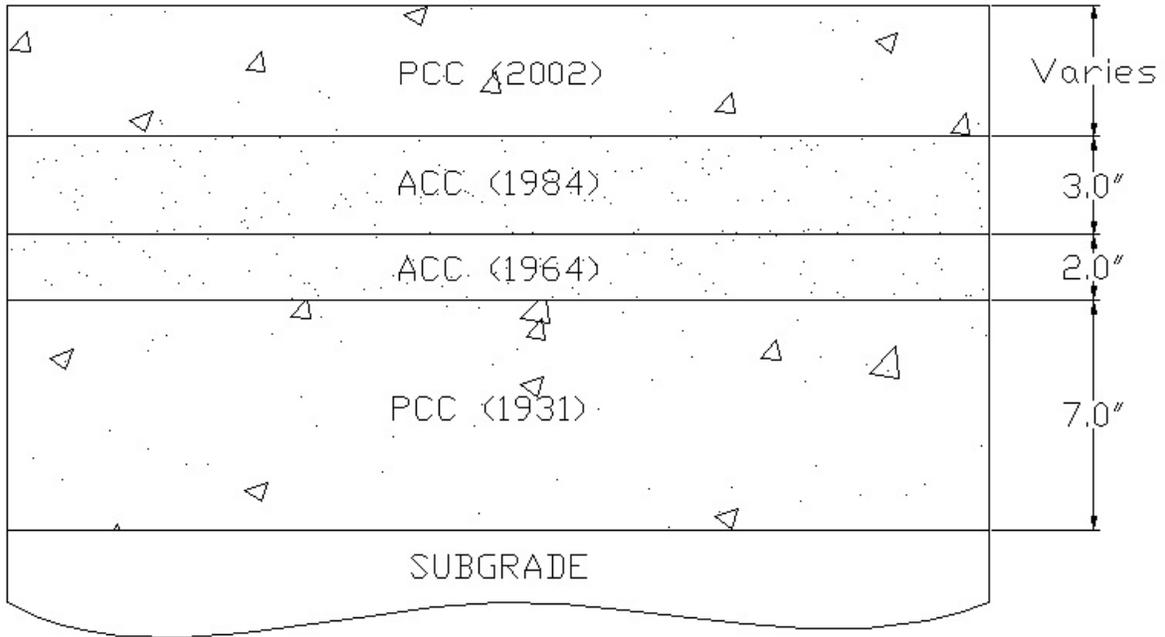
**Figure 2. Pavement Layers and the Dates of Construction**
