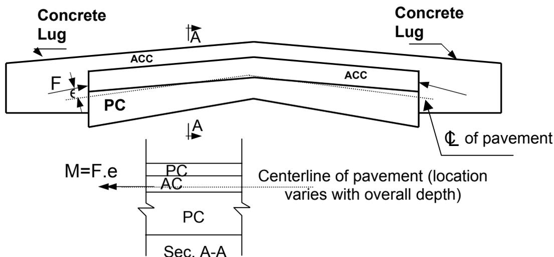
**Figure D.10. Schematic Showing Forces Acting on Composite Pavement, Effect of Crack (Joint) Depth**
