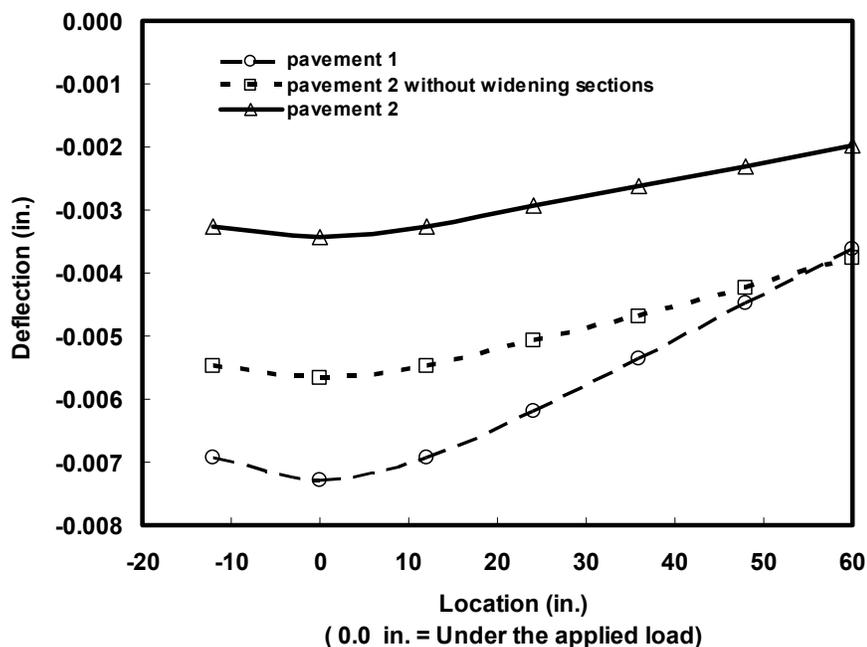
**Figure D.6. Comparison between Field and Analytical Results for Pavement 2 without the Two Widening Units (FWD Applied Near the Edge)**
