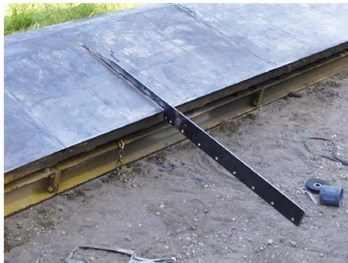
**Figure 11. Longitudinal Joint Forming Knife**
