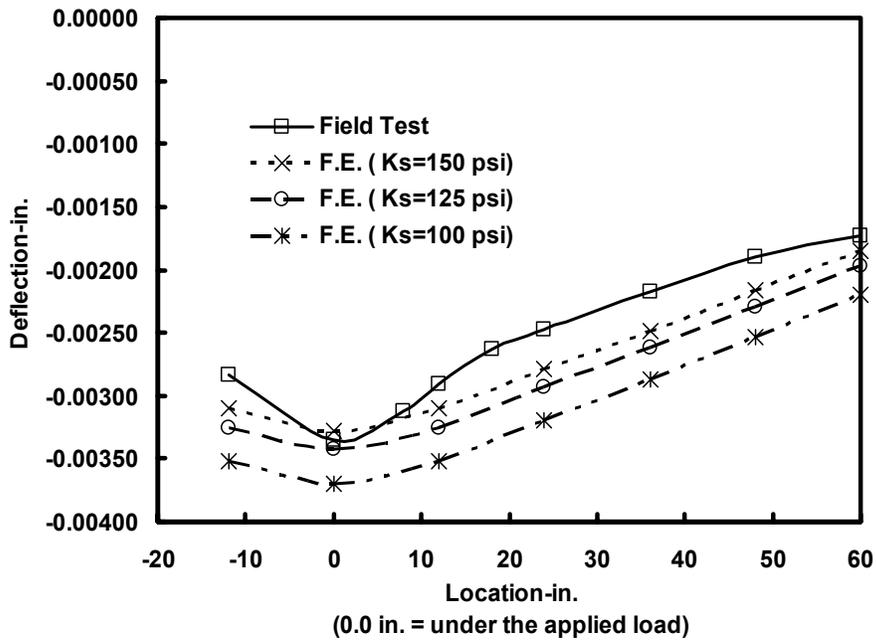
Figure D.5. Comparison between Field and Analytical Results for Pavement 2 (FWD Applied Near Edge)
