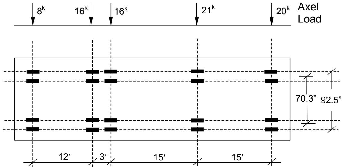
Figure D.7. Configuration of Truckload Used in Analysis
