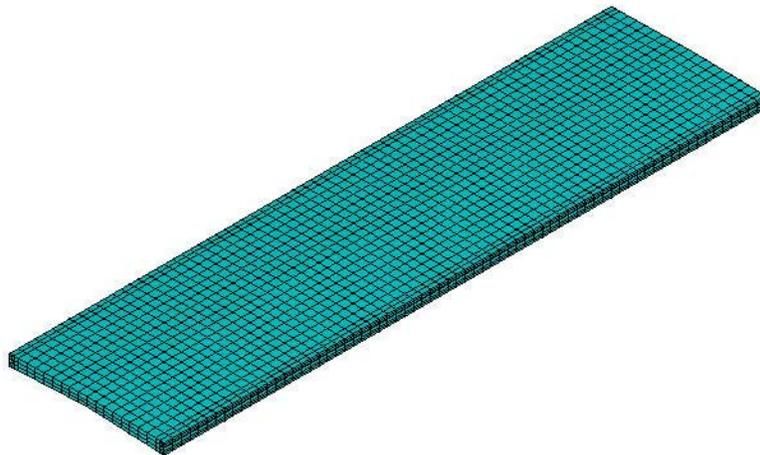
**Figure D.2. Isometric View of Pavement 1 Finite Element Model**
