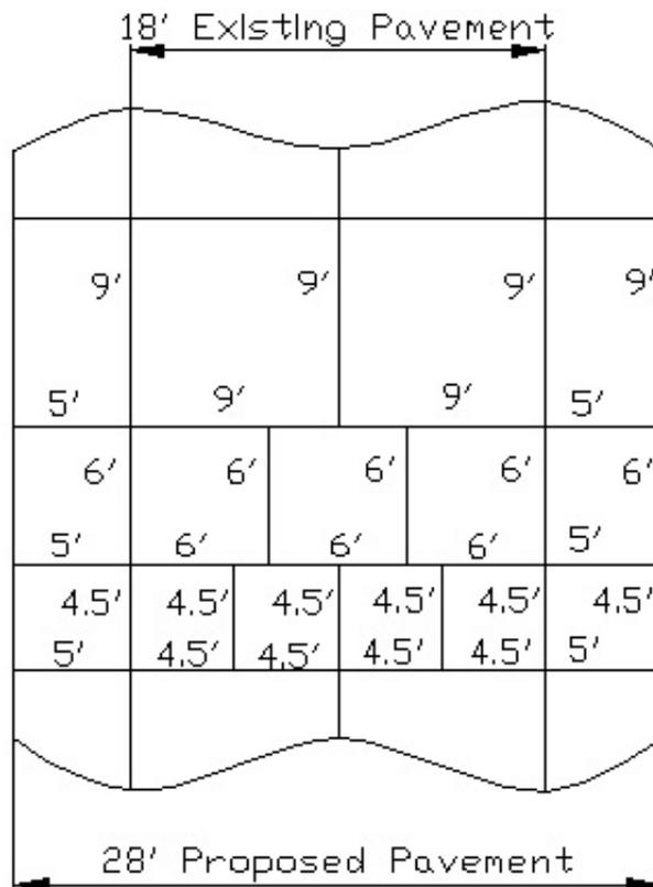
**Figure 12. Typical of Panel Sizes**
