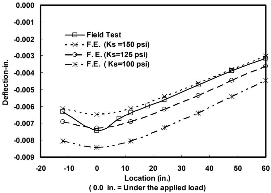
Figure D.4. Comparison between Field and Analytical Results for Pavement 1 (FWD Applied Near Edge)
