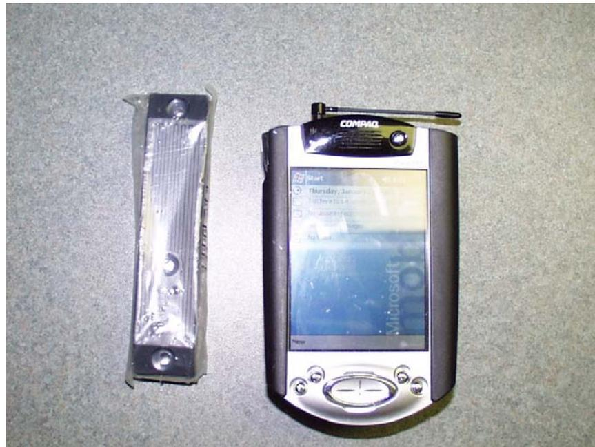
**Figure A.6. IRD Concrete Maturity Monitor (International Road Dynamics)**
