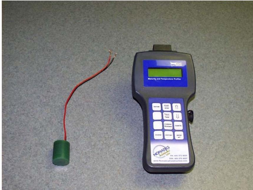
**Figure A.7. IntelliROCK System (Nomadics Construction Laboratory)**
