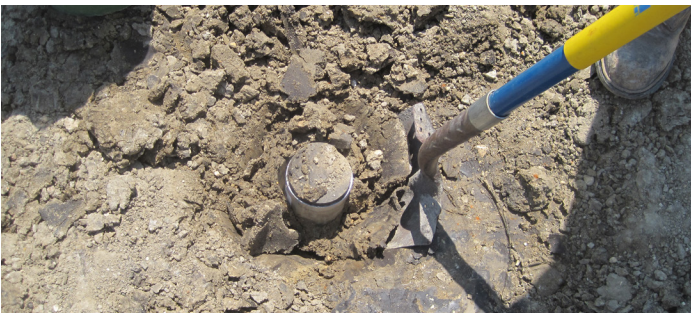
Figure 4. Drive core testing
