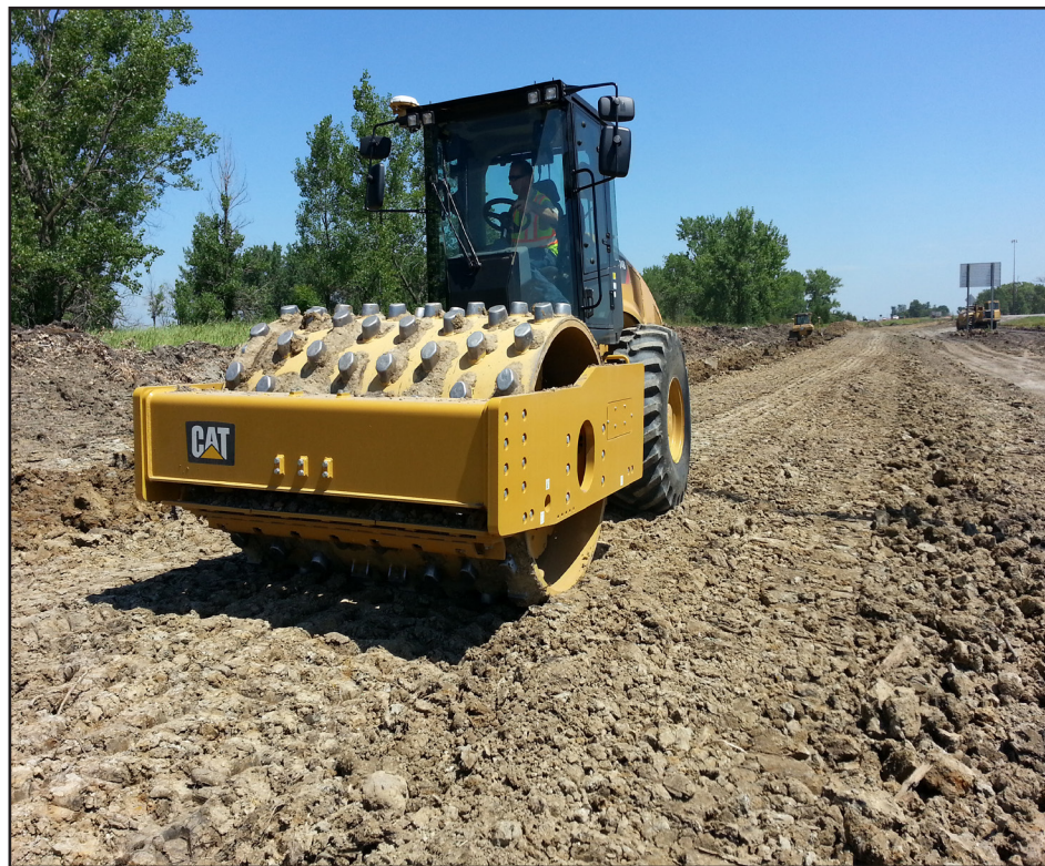
Figure 1. Caterpillar CS74B smooth drum roller with pad foot shell kit
