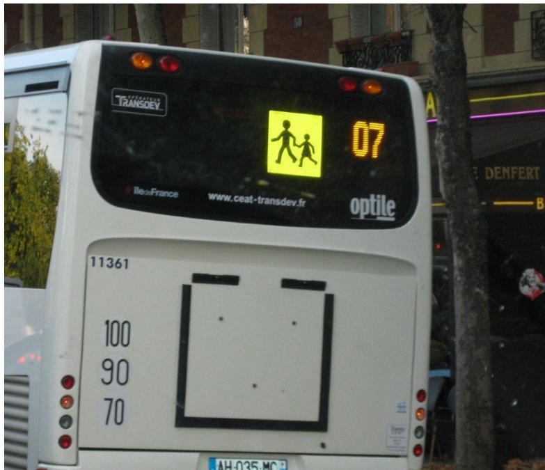
Figure 6. Transit bus with electronic sign display for loading and unloading in Paris, France (S. Chrysler 2011)
