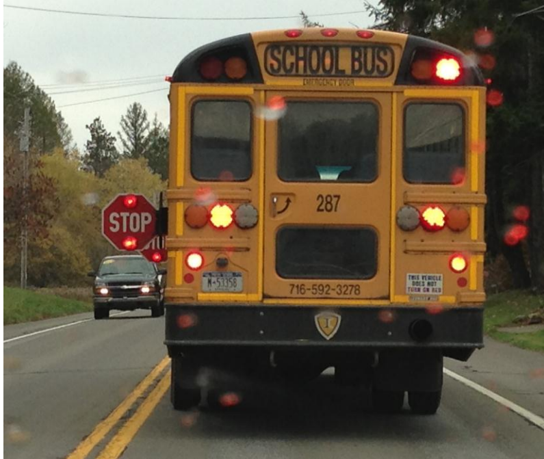
Figure 5. School bus in Buffalo, New York with additional rear stop arm (N. Hawkins 2012)
