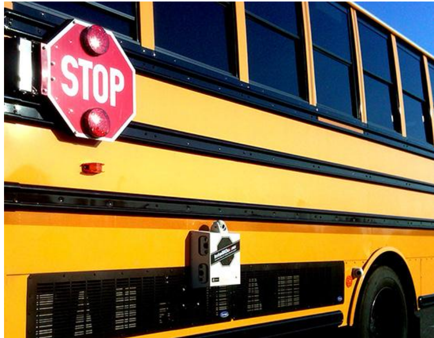
Figure 7. Stop-arm violation camera (Gatekeeper Systems Inc.)
