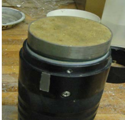
Figure 34. Intact soil sample and soil cutter placed upon sensor plate for moisture measurement
