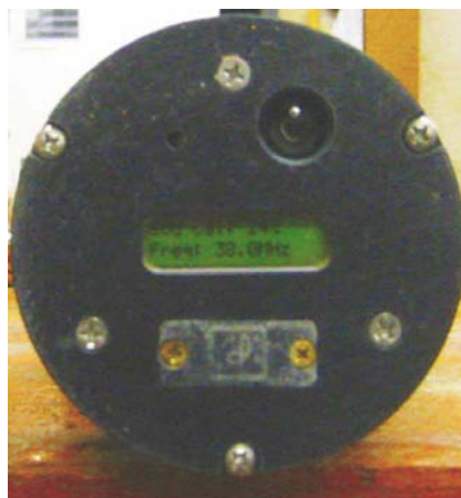
Figure 33. Frequency and calibration moisture content are displayed on the base of the electronics housing
