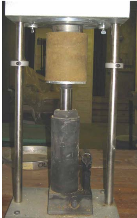
Figure 30. Use of a soil extruder and soil cutter to extract a sample for moisture measurement
