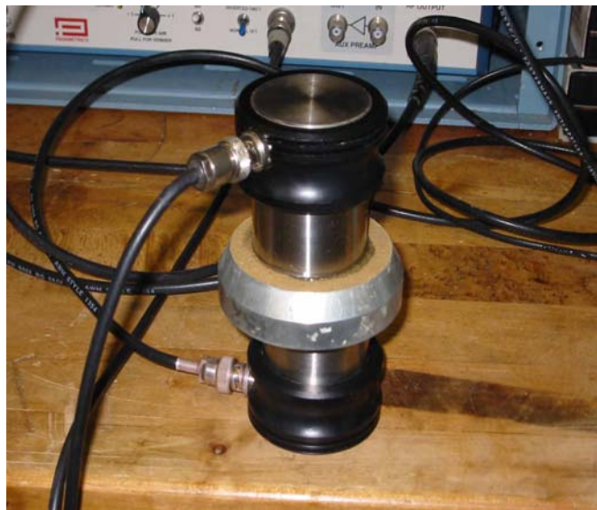
Figure 16. Experimental setup for measuring arrival times through soil sample
