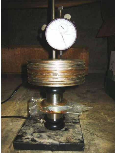
Figure 18. Apparatus for measurement of arrival time and settlement
