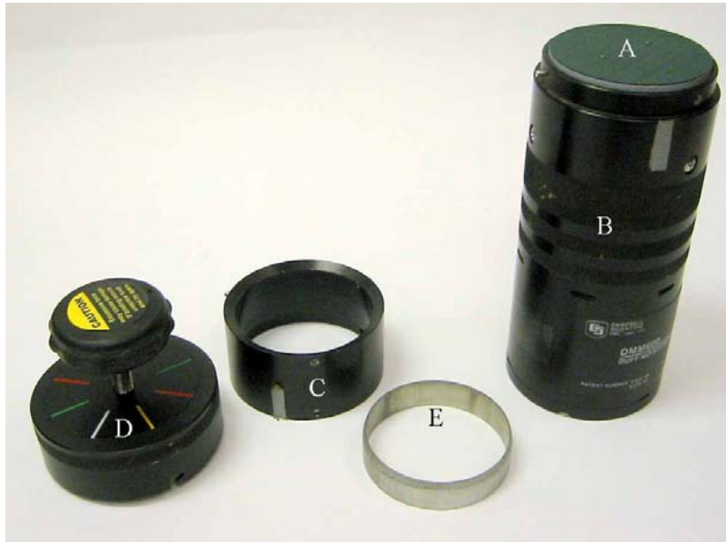
Figure 29. DMM600 components: (A) sensor plate / waveguides, (B) electronics housing, (C) sample chamber, and (D) sample chamber cap including compression knob (right) and compression plate
