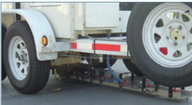
FWD equipment used to test and monitor trench restoration performance
