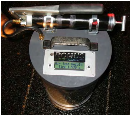
Figure 3.3 Schematic and Illustration of the ROMUS Air Permeameter
