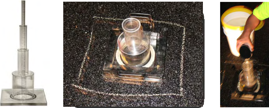
Figure 3.5 NCAT Water Permeameter
