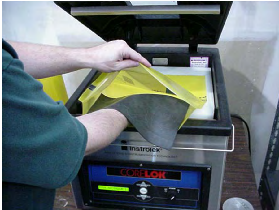
Figure 3.8 Instrotek's CoreLok Test Device
