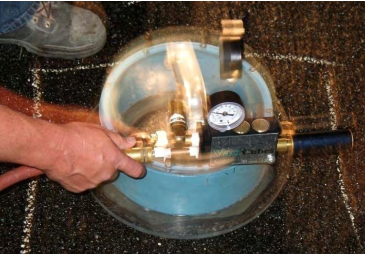
Figure 3.4 Kentucky Air Permeameter
