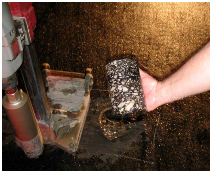
Figure 3.7 Removal of Core
