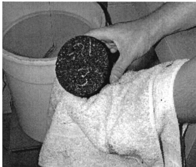
Figure 2.1 Blotting an HMA Specimen Dry (Indiana DOT, 2006)
