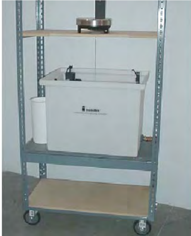
Figure 3.9 AASHTO T166 Test Configuration
