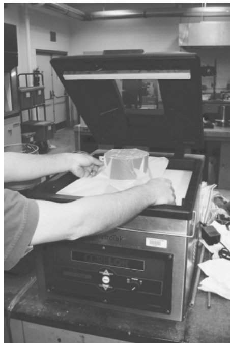
Figure 2.3 CoreLok Vacuum Sealing Device (Buchanan and White, 2005)
