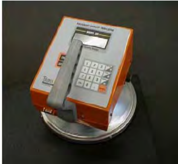
Figure 2.5 Pavement Quality Indicator
