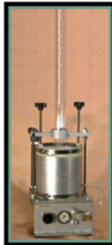
Figure 3. 10 Karol-Warner Flexible Wall Permeameter
