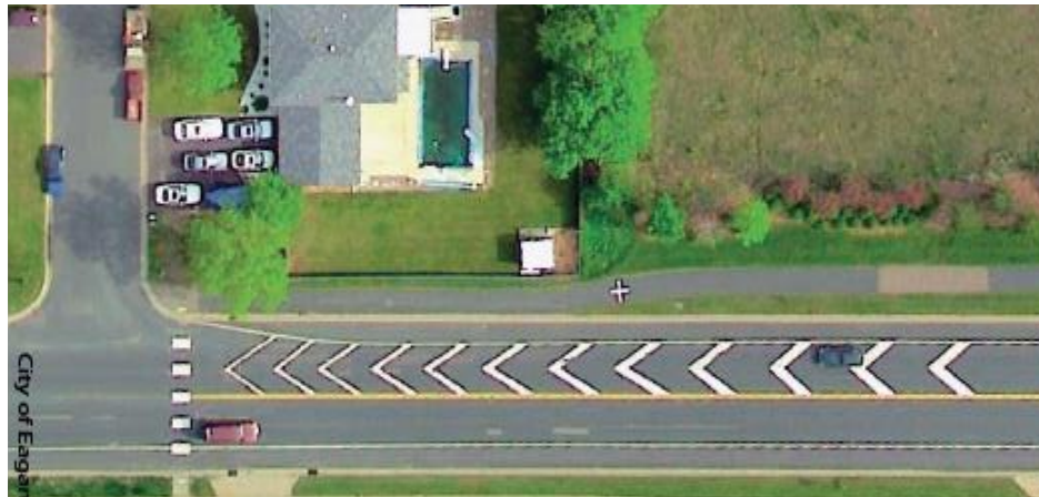
Figure 38: Aerial view of chevron lane markings in Eagan, Minnesota (Corkle et al., 2001)
