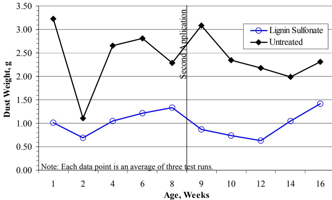
Figure 6.1.4. 260<sup>th</sup> Street 16 week lignin sulfonate dust measurement results.
