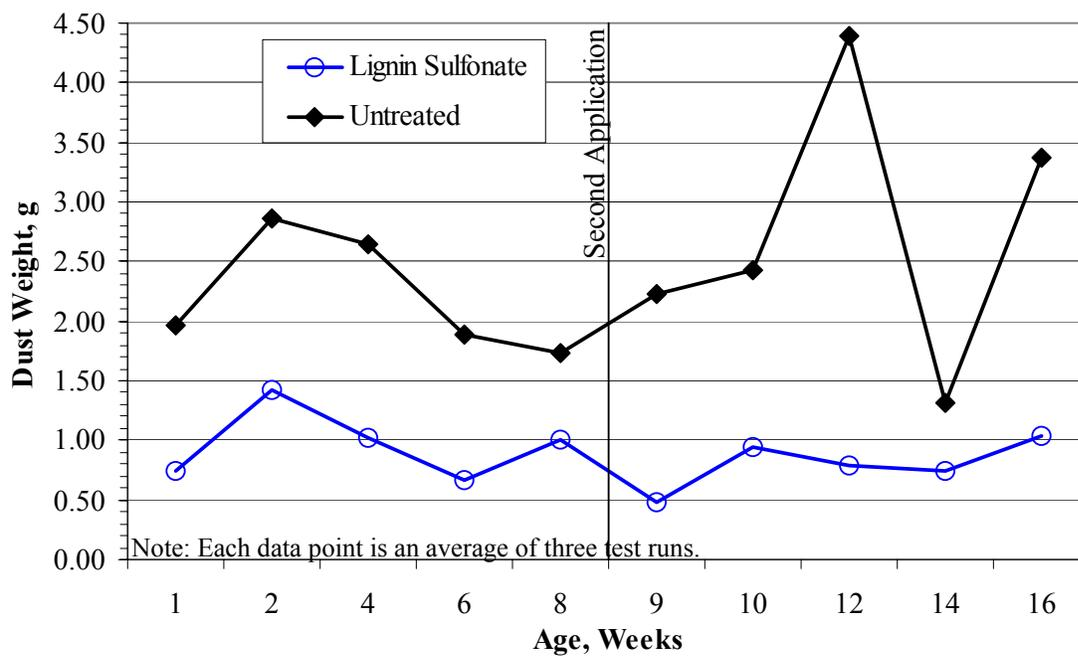
Figure 6.1.7. South 530<sup>th</sup> Avenue 16 week lignin sulfonate dust measurement results.
