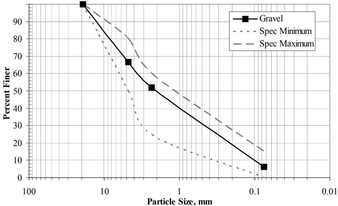
Figure 3.3.1. Gradation test results for virgin gravel.
