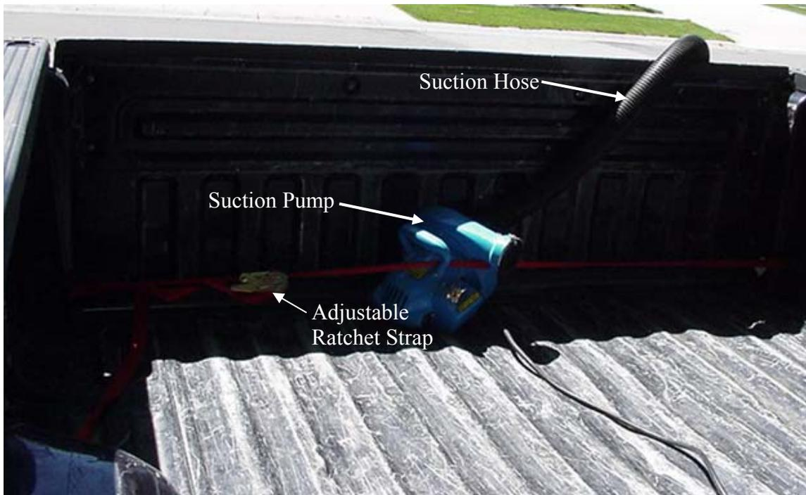
Figure 5.1.2. Suction pump secured by adjustable ratchet straps.
