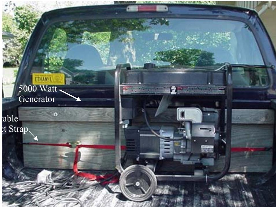
Figure 5.1.3. Generator secured by adjustable ratchet straps.
