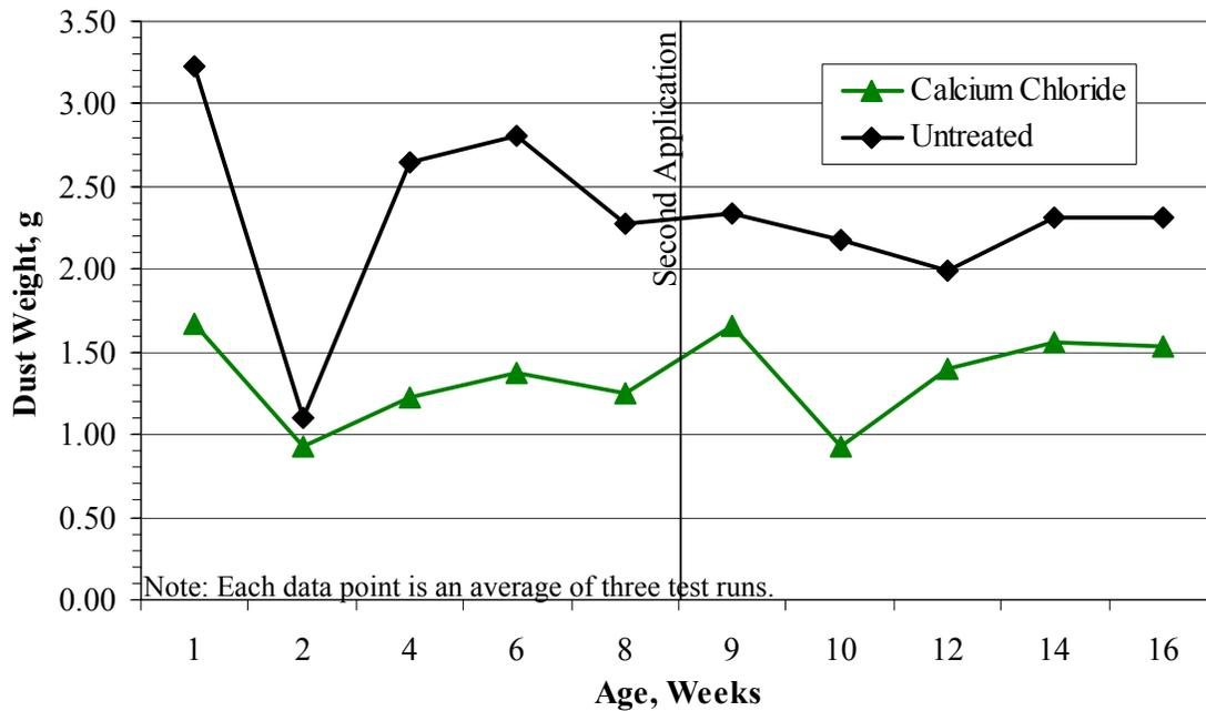
Figure 6.1.5. 260<sup>th</sup> Street 16 week calcium chloride dust measurement results.
