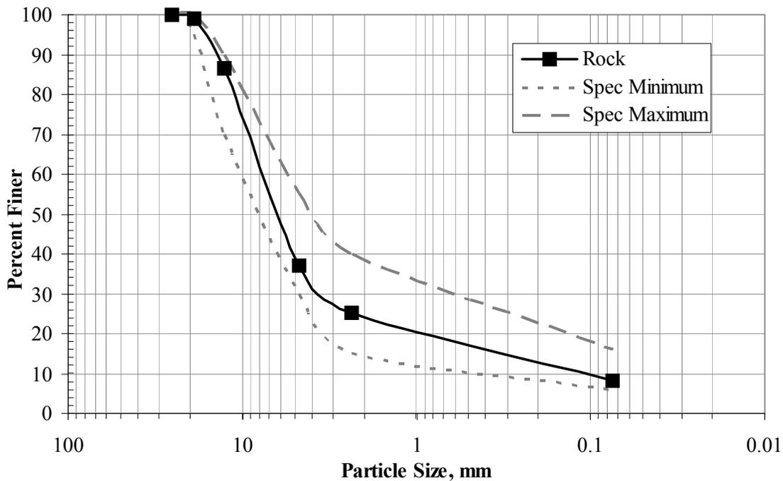
Figure 3.3.2. Gradation test results for virgin rock.
