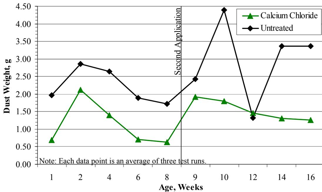
Figure 6.1.8. South 530<sup>th</sup> Avenue 16 week calcium chloride dust measurement results.
