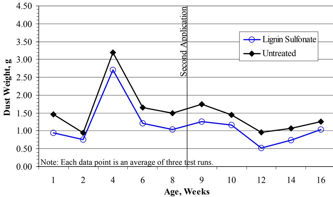
Figure 6.1.10. Grant Avenue 16 week lignin sulfonate dust measurement results.
