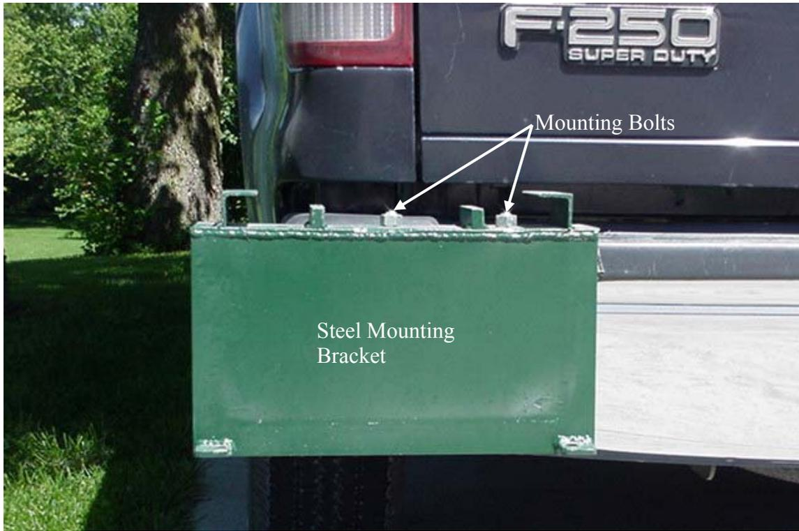
Figure 5.1.1. Steel mounting bracket and mounting bolts.
