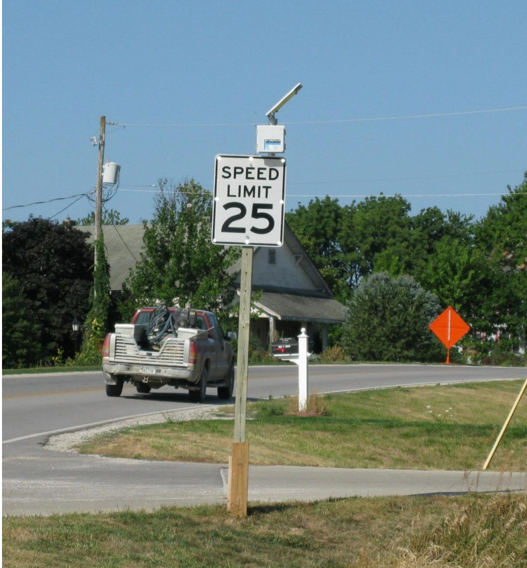
Figure 5-17: Radar-activated LED speed limit sign at east St. Charles community entrance
