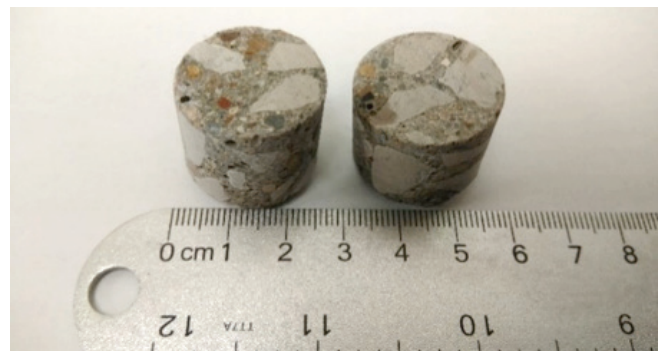
One-inch core plugs taken from the hardened concrete samples for use in mercury intrusion porosimetry tests
