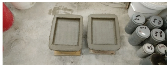
Slabs made from the concrete mixes for use in salt ponding tests
