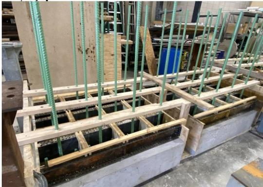
**Installing 0.5 in. divider to form discontinuous samples**
