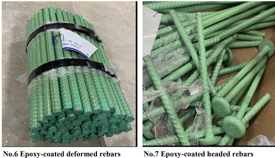
**Figure 11. Epoxy-coated rebar**
