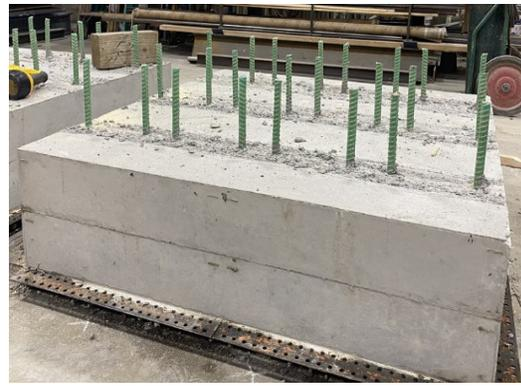
**Readied concrete slabs with embedded rebars**
