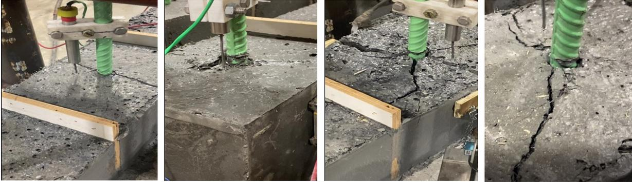
**Transverse splitting failure (TS)**
