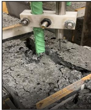
**Longitudinal splitting failure (LS)**
