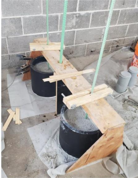
**Pull-out test samples during casting**
