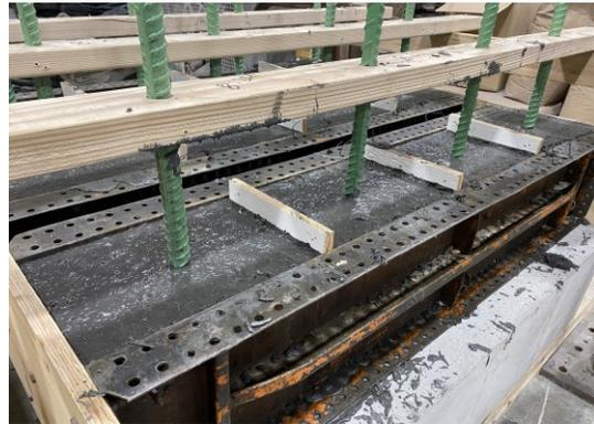
**Specimen after pouring UHPC**
