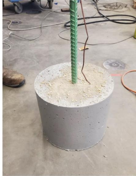
**Pull-out test sample after casting**
