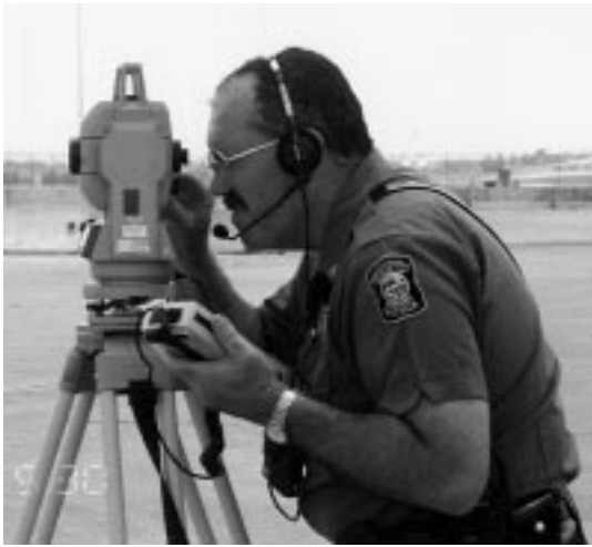
FIGURE 5 CHART officers measuring mock accident scene with total station.
