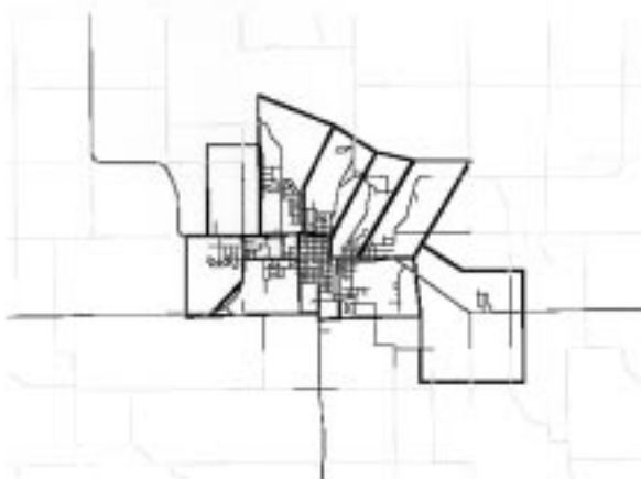
FIGURE 4 Traffic analysis zones developed for Waverly, Iowa.
