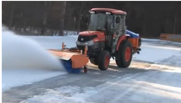
Figure 16. Rotary snow brooms efficiently remove snow from uneven surfaces.
