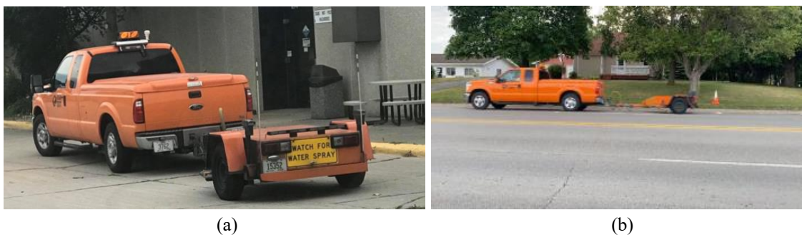
Figure 19. Locked-wheel skid tester: (a) close-up view and (b) in operation
